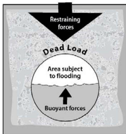
Figure 1. Tanks are typically buried 3 to 4 feet below finished grade to provide adequate slope for piping and protection from traffic loads. Except in areas with high water tables or areas subject to flooding, the weight of the backfill and pavement over the tank is sufficient to offset buoyance and prevent flotation.
